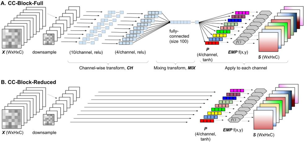
Figure 2: A fully expanded *CC-block*(top). Solid lines are learned layers and dashed are data-flow. **CH** is composed of 2 hidden layers, each applying a fully-connected layer to *each* channel independently. **S** is then multiplied by  $X$  to produce the output. Bottom: Reduced *CC-block* that uses neither **CH** nor **MIX**. Experiments will be conducted with both A & B.
