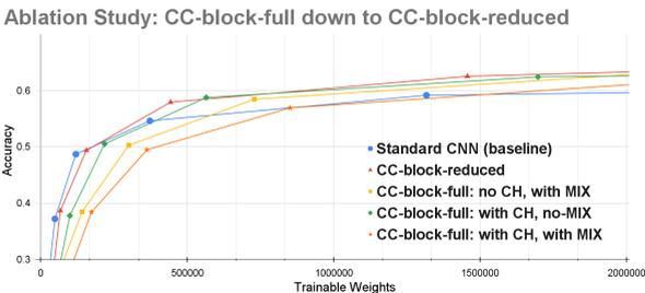
Figure 6: Ablation study. Three versions of *CC-block-Full*: (a) with *CH* and *MIX*, (b) without *MIX*, and (c) without *CH*. *CC-block-Reduced* is also shown; from Figure 2(B).
